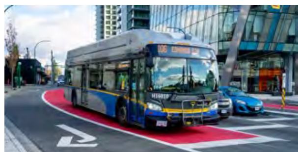
Bus priority lanes, such as this queue jump lane at Edmonds Street in Burnaby, help buses avoid congestion, improving reliability for transit customers
