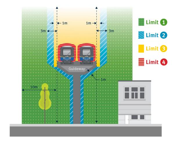
Note: The drip-line is a line which extends from the edge of the guideway (or walkway) to the ground below. The area of SkyTrain's concern extends from below ground up to and beyond the guideway due to the dangers of falling objects into the track from above or to underground structures such as footings, caissons, or tunnels.
