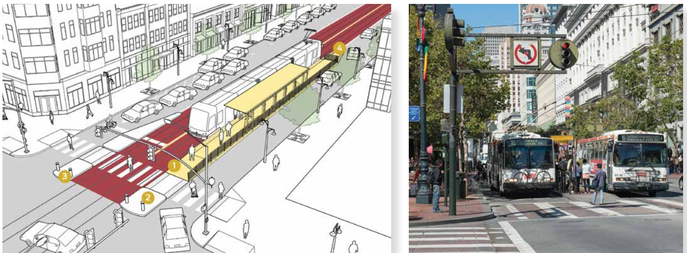
Figure C1.2: In-Street Boarding Island Stop
