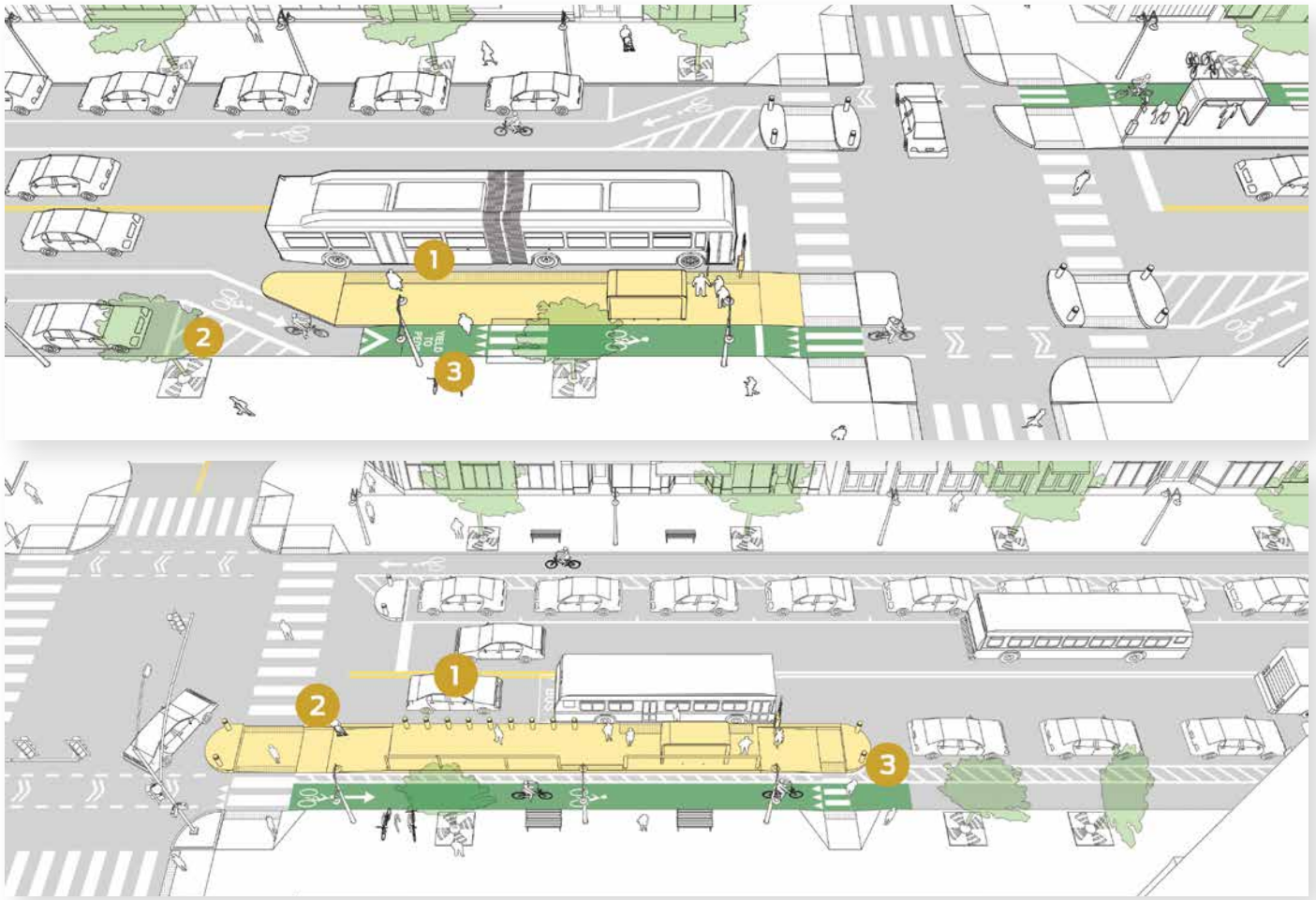
Figure C1.1: Near & Far-Side Boarding Island Stops
