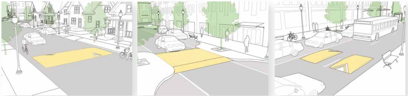
Figure C3.1: Vertical Control Devices – Speed Hump (Left), Speed Table (Middle), and Speed Cushion (Right)
