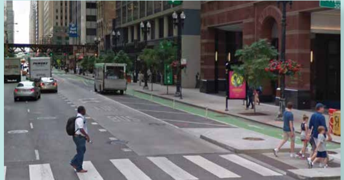
Figure C5.4: End of Transit Approach Lane with Separated Turning Traffic – Washington Street in Chicago 2
