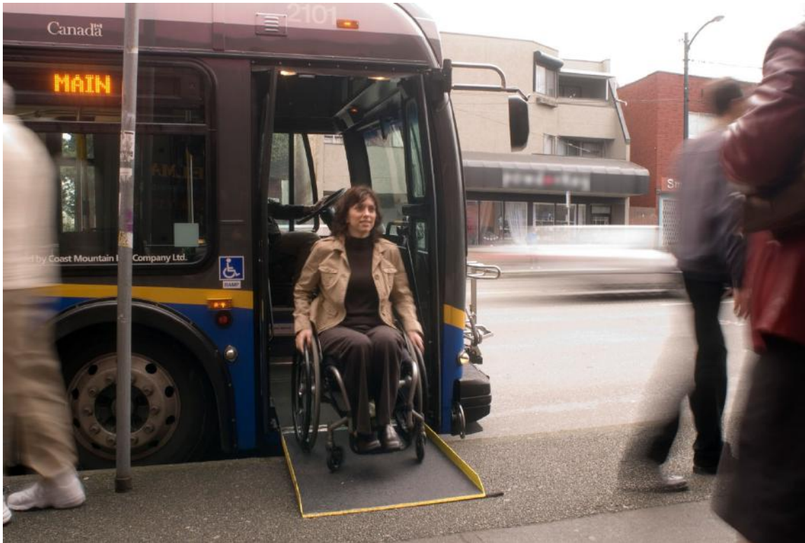
Figure 1.7.2 Typical wheelchair ramp
