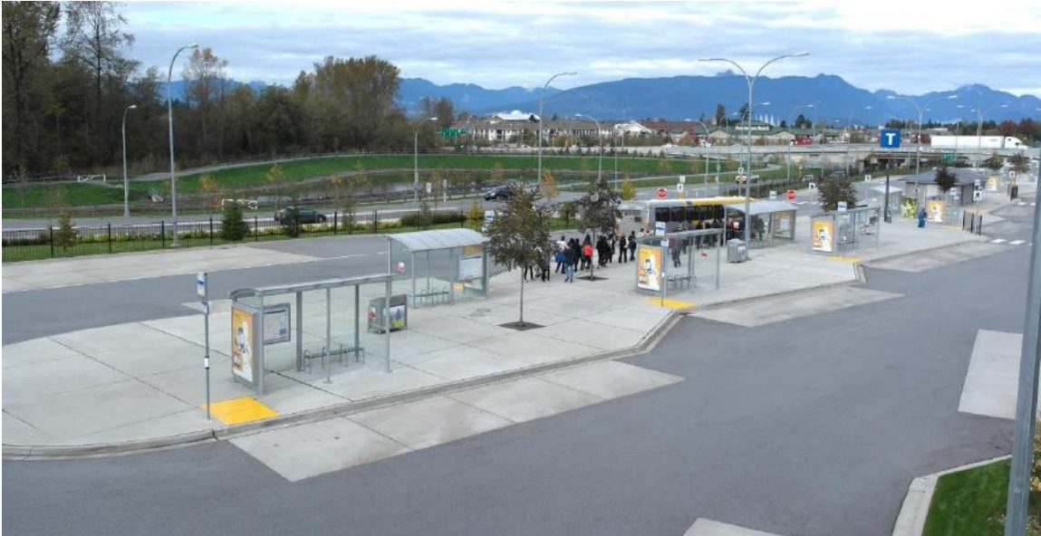
Figure 3.4.8 Example of sawtooth bus bays
