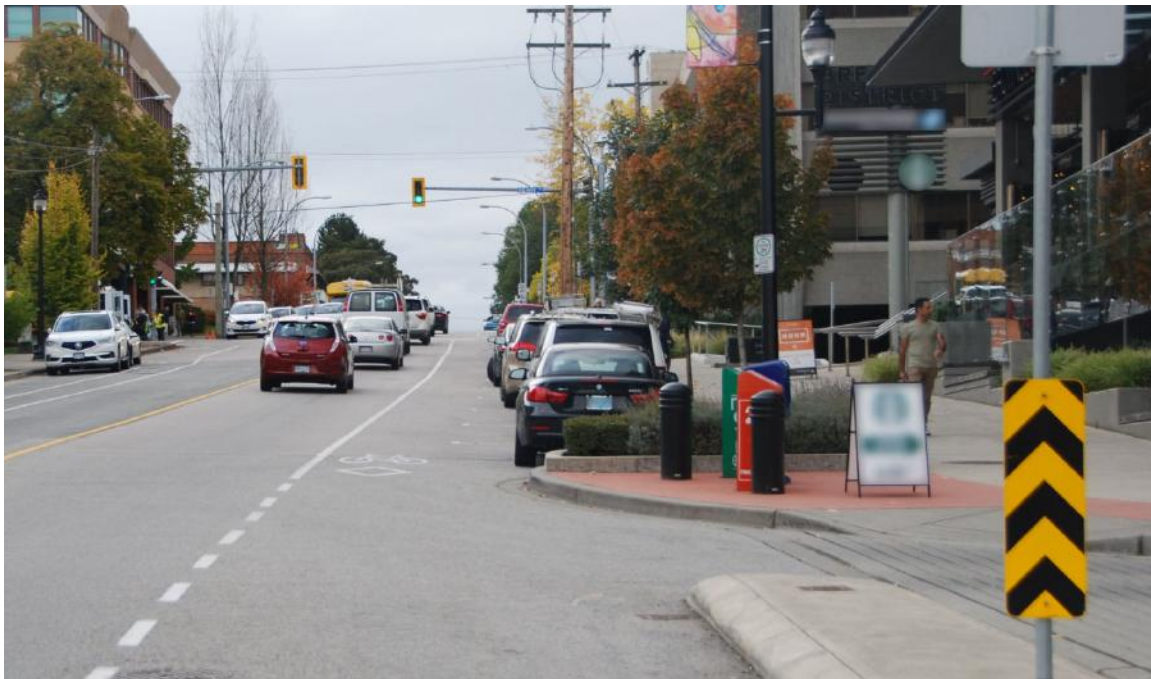
Figure 2.7.2 Example of curb extension
