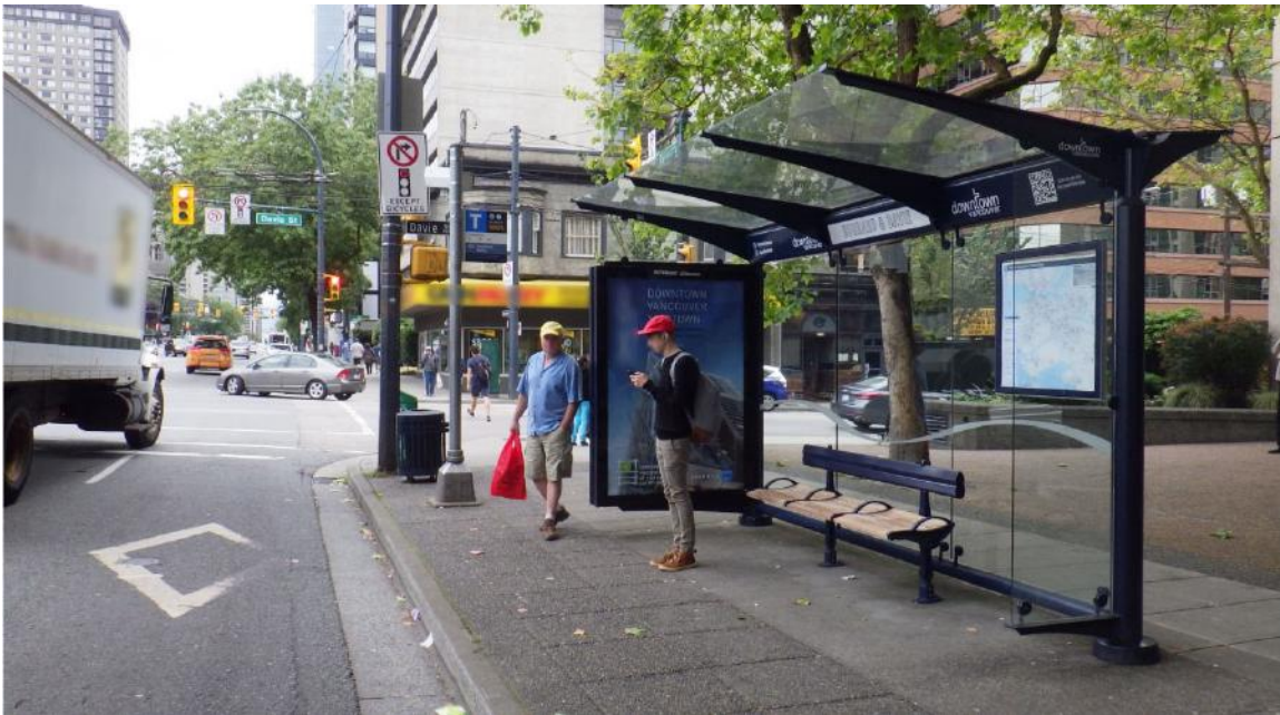
Figure 3.3.5 Example of near-side bus stop
