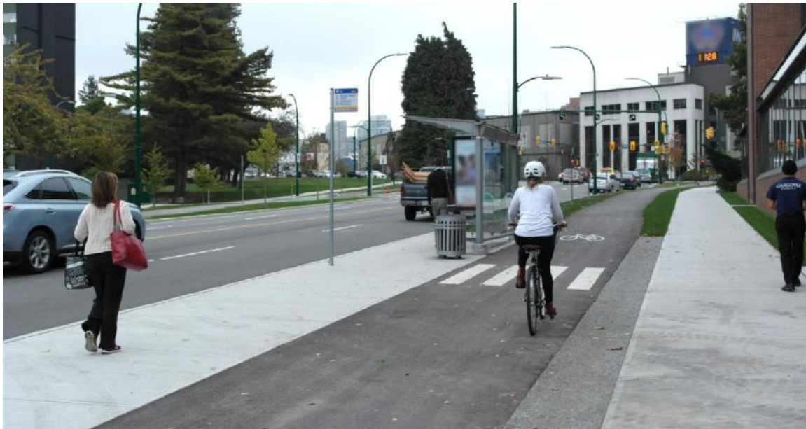
Figure 3.4.15 Example of island bus stop
