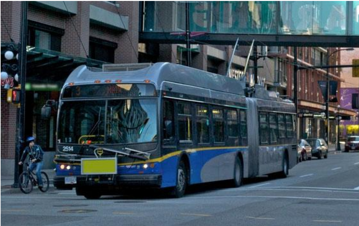
Figure 1.2.4 Articulated trolley bus
